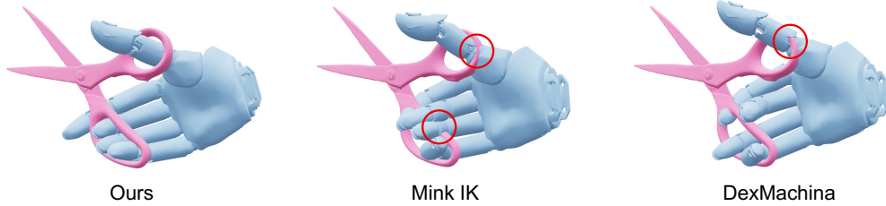
Figure 5: Qualitative Retargeting Results. Sample retargeted configurations produced by our method, Mink IK, and DexMachina for the WUJI-Scissors task. Our method produces a human-like grasp that preserves the hand-object interaction semantics, while the other two baselines produce physically implausible or unstable grasps that are not suitable for RL training. The red circles highlight significant hand-object penetrations.
